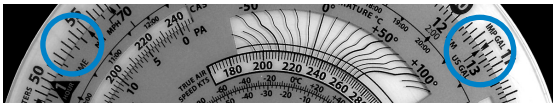
Figure 6. Align the US GAL and IMP GAL arrows to convert between these units.
