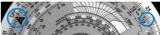
Figure 11. Set elapsed time under distance then read ground speed above the time index.
