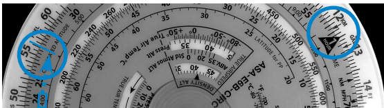
Figure 10. Place the time index under ground speed, find fuel endurance on inner scale, then read distance opposite this number on the outer scale.
