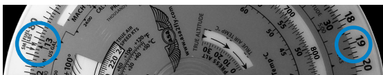
Figure 7. Place Fuel LBS arrow above US GAL arrow and read the weight of fuel above total gallons.
