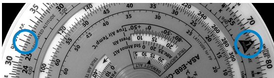
Figure 13. Set time flown opposite gallons and read fuel rate above the rate arrow.
