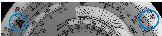
Figure 19. Set distance flown on middle scale opposite off-course distance and read correction above the rate arrow.
