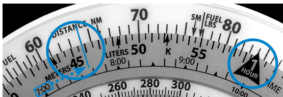
Figure 12. Point rate index to fuel consumption, find fuel capacity on outer scale and read fuel endurance below.
