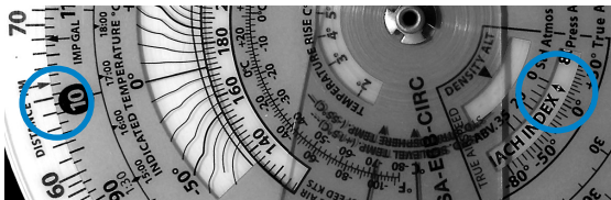
Figure 16. Set double-pointed MACH INDEX at outside air temperature and read true airspeed on the white disk above the Mach Number on the blue disk.
