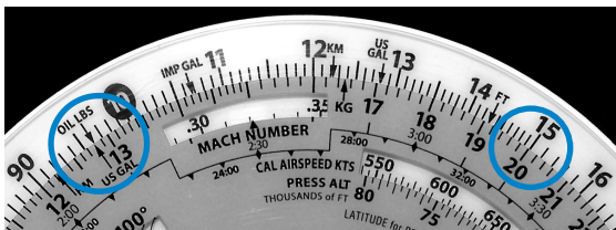
Figure 8. Place Oil LBS arrow above US GAL arrow then read weight of oil above total gallons.
